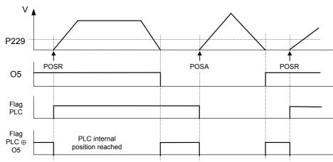
The PLC marker is toggled when a positioning command is transmitted. The "EXCLUSIVE-OR" operation of the PLC marker and output O5 can be processed as a PLC-internal "Position reached" message.
